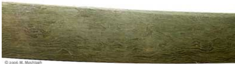
Figure 3 : Rose pattern on the blade surface of a shamshir (above)
