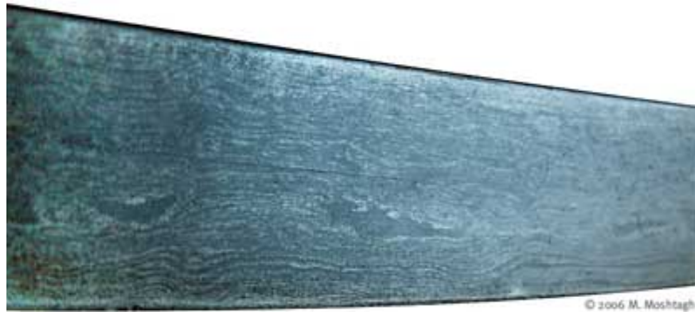
Figure 5 : Sham pattern on the blade surface of a shamshir (above)
