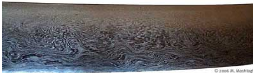
Figure 3 : Rose pattern on the blade surface of a shamshir (above)
